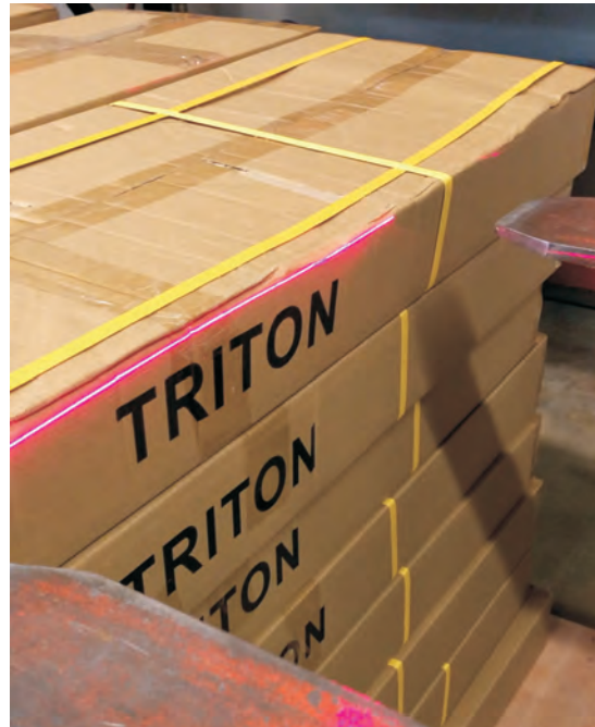
BRIGHT RED LASER LINE SHOWS FORK TINES POSITIONING
